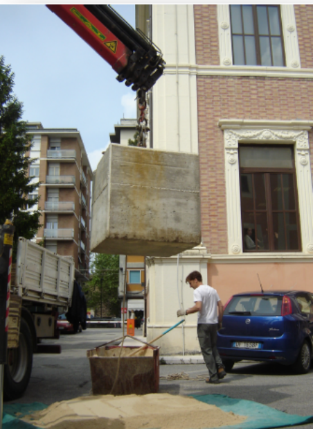
Dynamic shaking test by impact of r.c. cube
